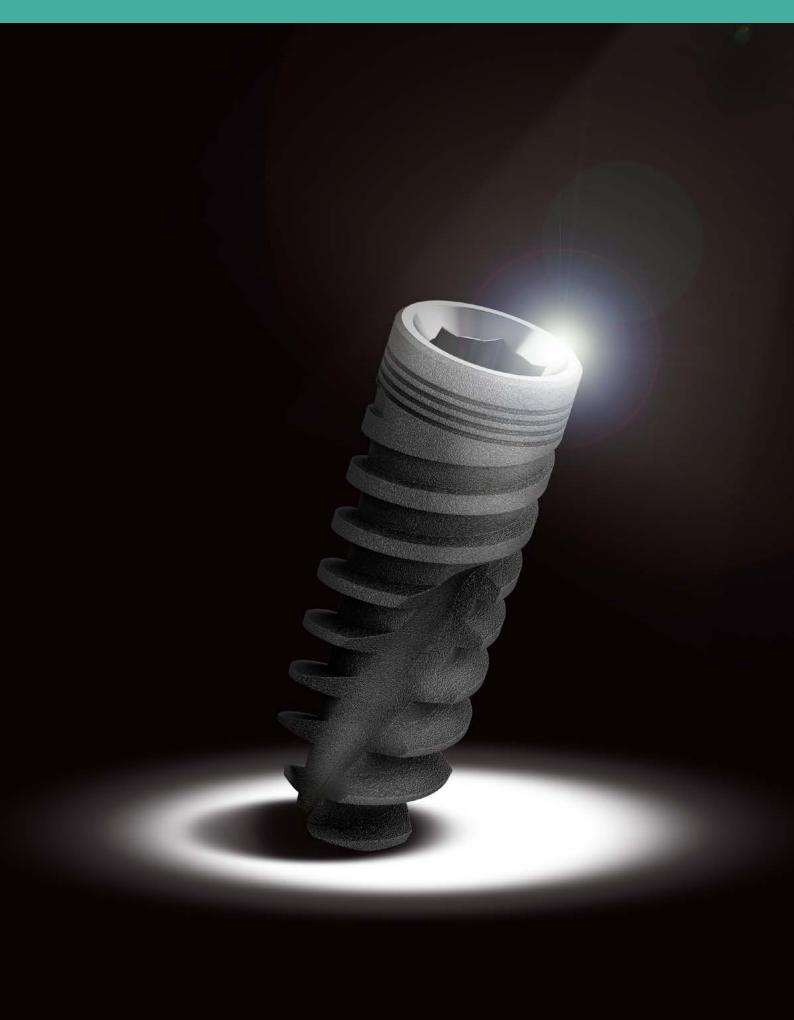
BiotecSPTT implants share the same three-thread zone concept asSPRimplants but they also incorporate platform switching in their design, which keeps the implant-abutment connection away from the bone, minimizes bone resorption and allows for more vital growth of the soft tissue.
